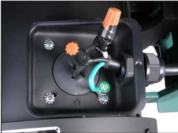
Figure 155. G0605X1/G0696X motor junction box.
